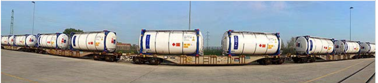
Figure 1. UN Portable T11 35,000 litres on rail. It is app. 55 t methanol on one railcar.
